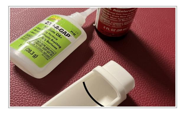
First put the glue adapter in this position. Than only glue a few! CA only from the inside at the <u>black</u> line.
