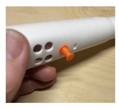
Push the lid in from the outside, glueing is not necessary. The lid sits tightly in the extension button.
